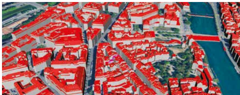
3D city model developed by the SECuRE project, showing photovoltaic energy potential on rooftops in Zurich.
